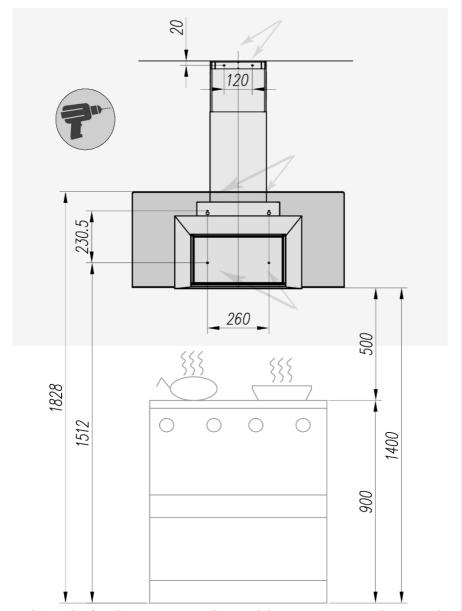
Hood must be fitted on minimum 5" Round ducting or rectangular equivalent
